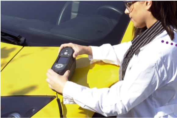
Gently place the spectrophotometer on the panel to be measured.
